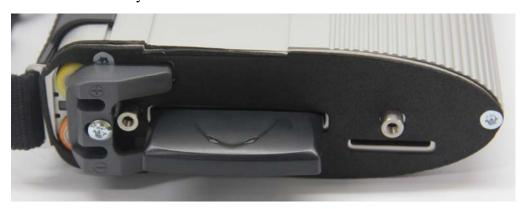
**4.3** Cover the rubber and fix the screws to finish all the work.
