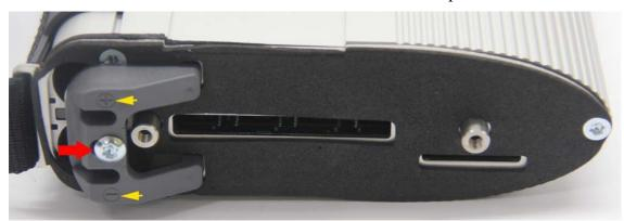
3.2 Take out the fixation of Batteries Space. Pay attention to the Battery polarity marked in the Batteries Space.
