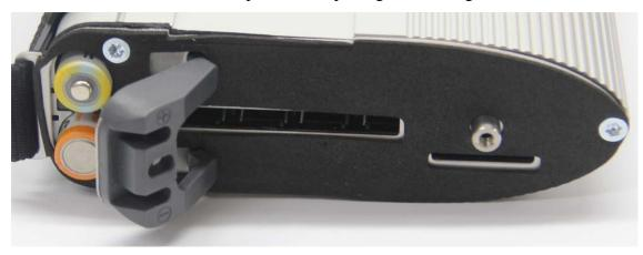
3.5 Use the T20 Plum screwdriver to fix the screws of Batteries Space fixation as below. Inserting the batteries is finished.
